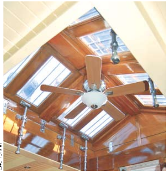
Called butterfly hatches due to their look when opened, each section can be lifted independently, with a choice of height adjustments.
